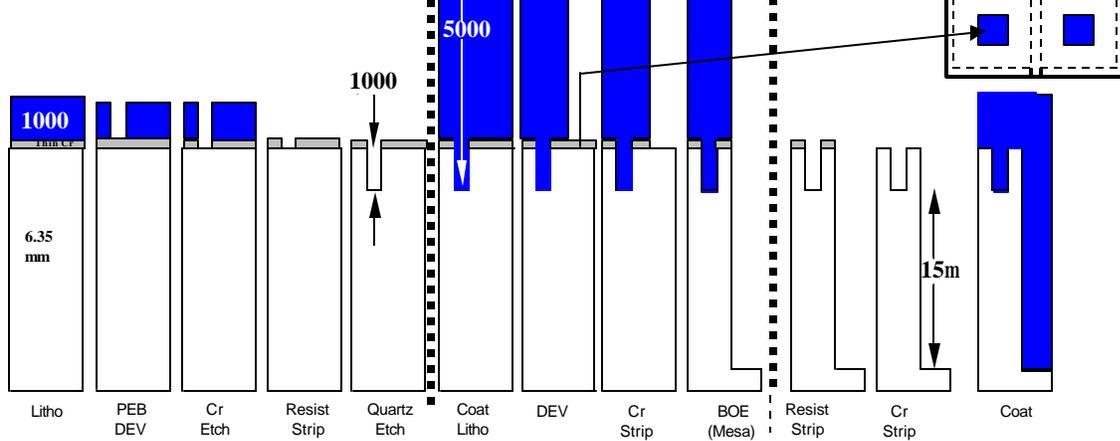
Figure 2. S-FIL analogous process route compared to a typical Chromeless PSM route
