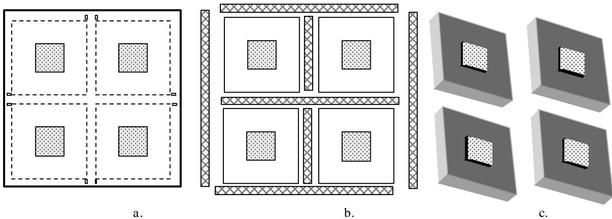
Figure 3 a) 6025 plate layout of four S-FIL pedestal templates. b) diced 6025 plate resulting in four templates and discarded quartz. c) four S-FIL templates, 65mm x 65mm x 6.35mm, with 25mm square raised (15µm) active (center) area.
