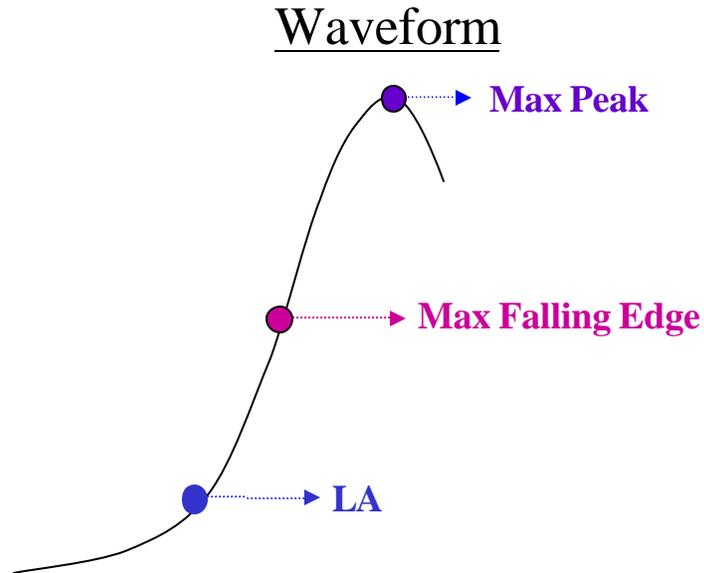
Figure 9. Available modes for topographic point detection
