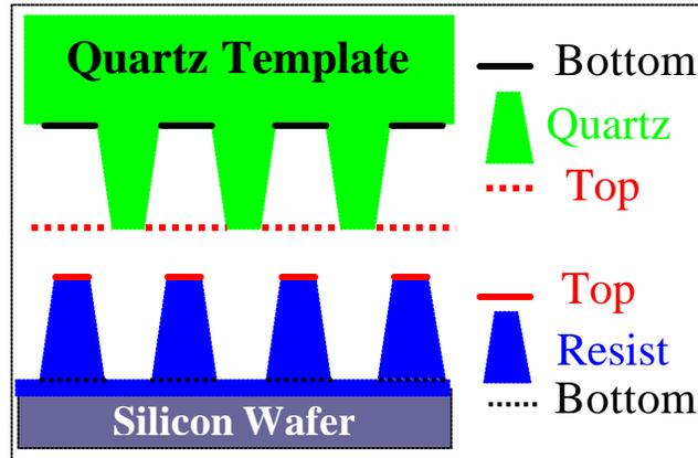
Figure 1. Template and imprinted wafer diagram
