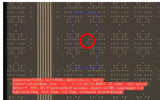
Resulting imprint repeating defect
