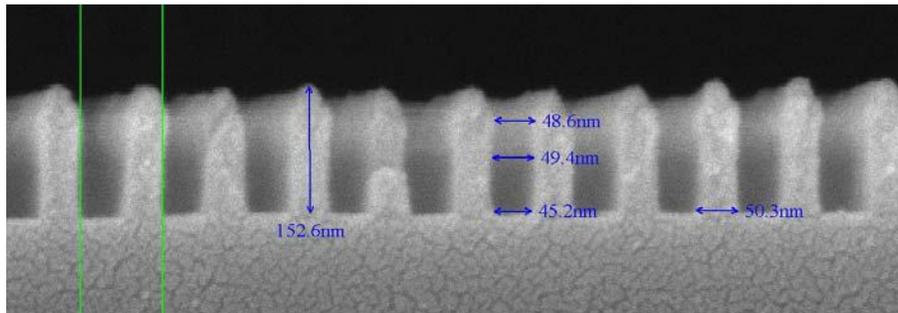
Figure 7. SEM micrograph of an 50 nm l/s pattern after dry developing an imprint. The critical dimension of the features is near that shown in the top down and cross section images of Figure 6.
