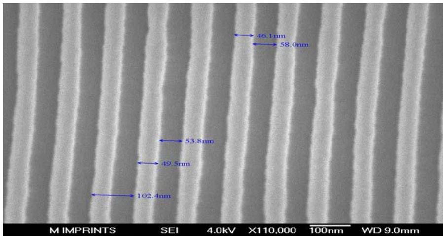
Figure 6. SEM micrographs of a cross section (top) of the 50 nm l/s imprint. The feature height is 60 nm, the residual layer is 40 nm, the transfer layer is known to be 60 nm and the critical dimension of the feature is near 50 nm. The top down SEM micrograph (bottom) shows a nearly 5 nm variation in the critical dimension for the pattern. This variation is mainly due to the line edge roughness of the template.
