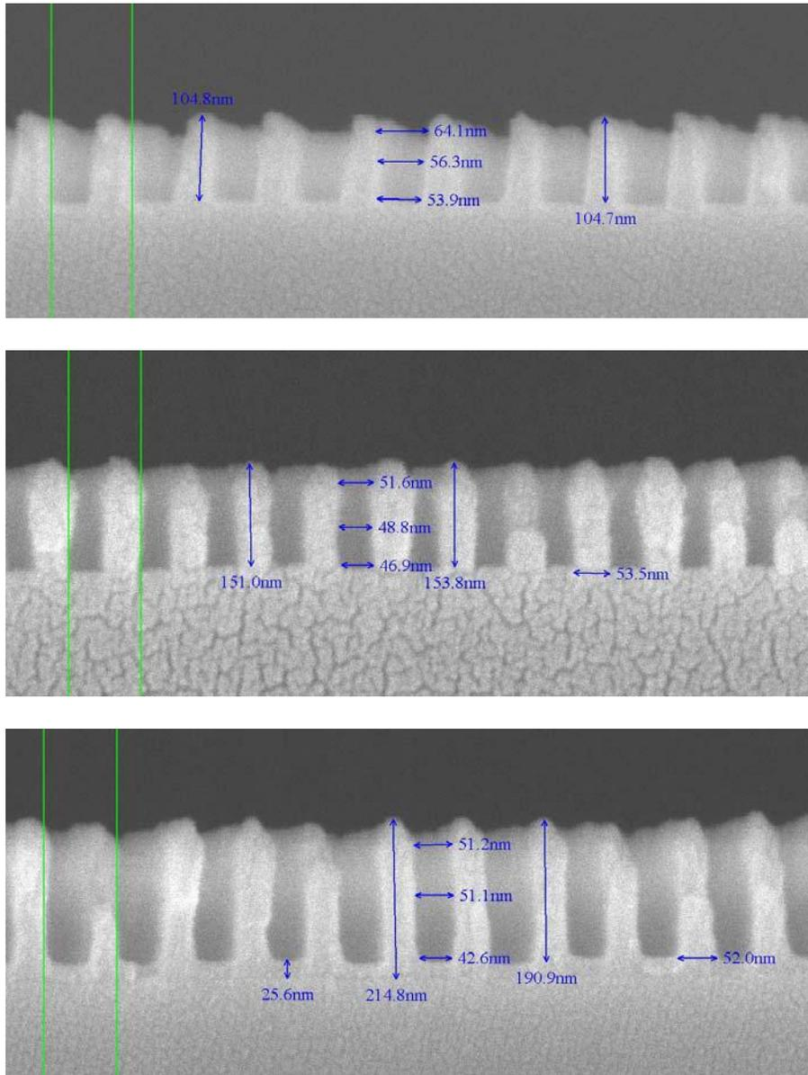
Figure 8. SEM micrographs of 50 nm l/s patterns after the dry develop step. The feature height variation is the result of intrinsic wafer height variations. The resist height variation of 114 nm is observed with a critical dimension near the calculated 5 nm window.
