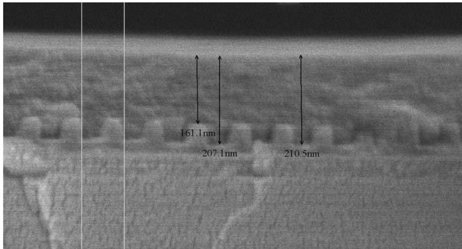
Figure 3: Spin-on planarization of imprint using Silspin. Silspin is a high silicon content spin on planarization material, which provides good etch selectivity to the underlying imprint and transfer layers.
