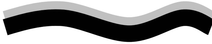
Figure 1: Substrate is coated using Brewer Science DUV30J as a transfer layer. A typical coating thickness of between 60 and 240 nm is used.
