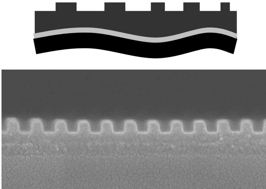
Figure 2: Imprint on transfer layer. The imprint layer on prime, double side polished lithography grade silicon wafers has a mean residual layer thickness of 60 nm and a tooth height of 60 nm.
