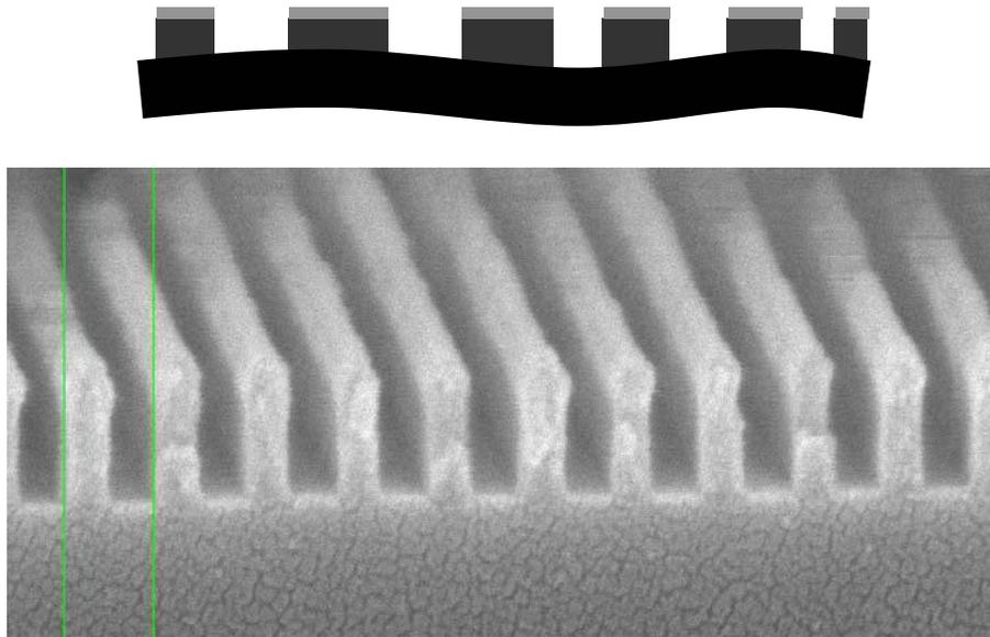
Figure 5: Final etch to define features. The imprint and transfer layers are etched down to the substrate using oxygen under anisotropic conditions.
