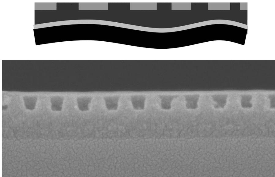
Figure 4: Breakthrough etch of Silspin planarization layer. The Silspin is etched back to reveal the tops of the imprinted features at which point the etch process is stopped.
