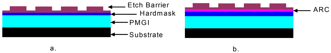
Figure 3. a) S-FIL material stack with no glue layer; b) S-FIL material stack with a glue layer
