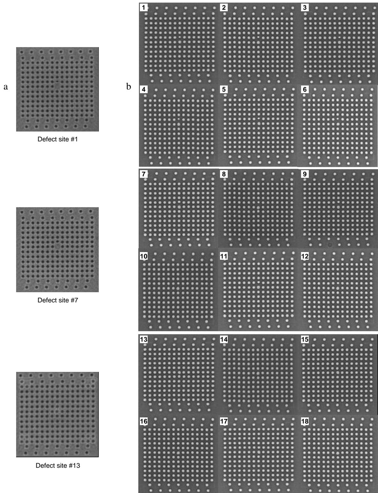
Figure 8. a) SEM image of repaired  $40 \times 40 \text{ nm}^2$  contact hole defects in the 40nm design. b) Imprint results after repair of 18 different arrays with identical defect size.
