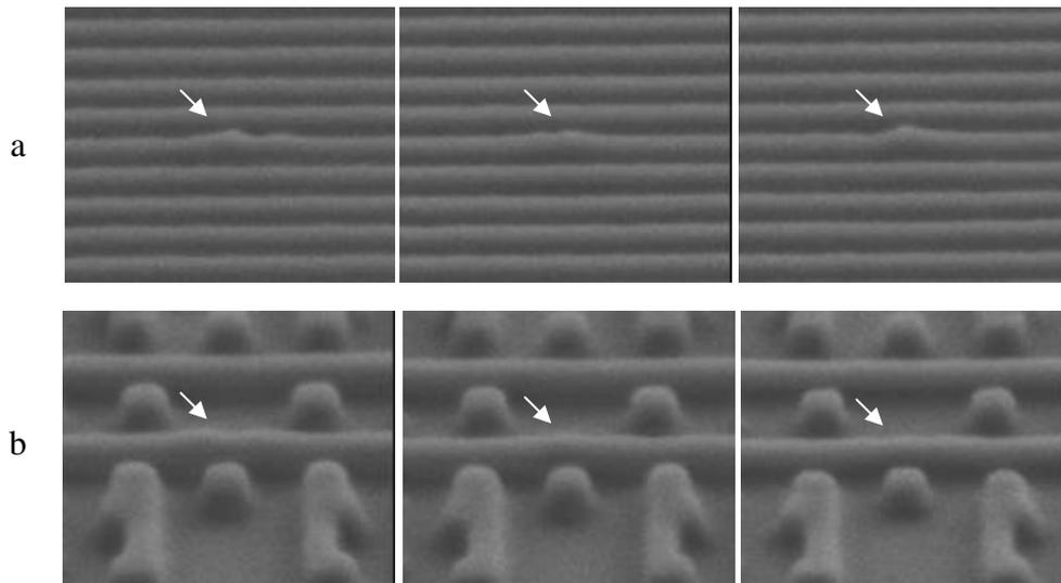
Figure 7. Tilted high-magnification images of imprints of repaired identical defects in the 40nm half pitch designs for three line/space patterns (a) and SRAM Metal 1 patterns (b).
