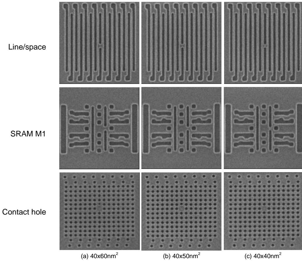
Figure 3. SEM images of programmed defects in the 40nm half pitch design on the template: a) line/space pattern, b) SRAM Metal 1 cell and c) contact hole array. In the contact hole design the smaller holes above the center defect appear due to the implementation of programmed defects larger than  $40 \times 40 \text{nm}^2$ .
