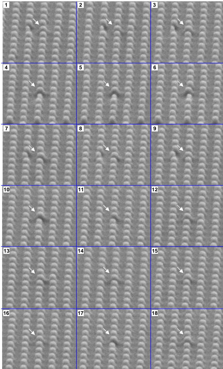
Figure 9. Imprinted pillar arrays after defect repair in the 40nm half pitch contact hole arrays on the template. All repaired pillars have equal shape and size and demonstrate the repeatability of the repair process.
