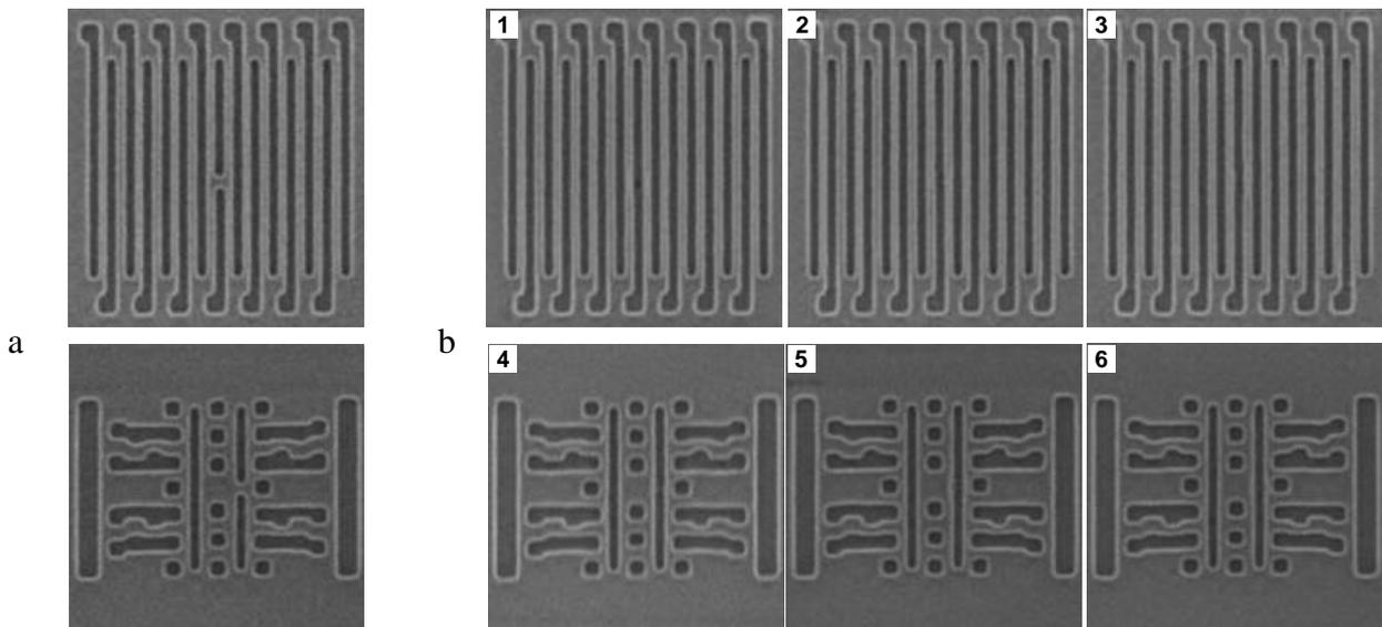
Figure 4. a) SEM images of a mousebite defect in the 40nm line/space and SRAM Metal 1 pattern before repair, b) SEM images of identical  $40 \times 50 \text{nm}^2$  mousebite defects after repair at three different locations.
