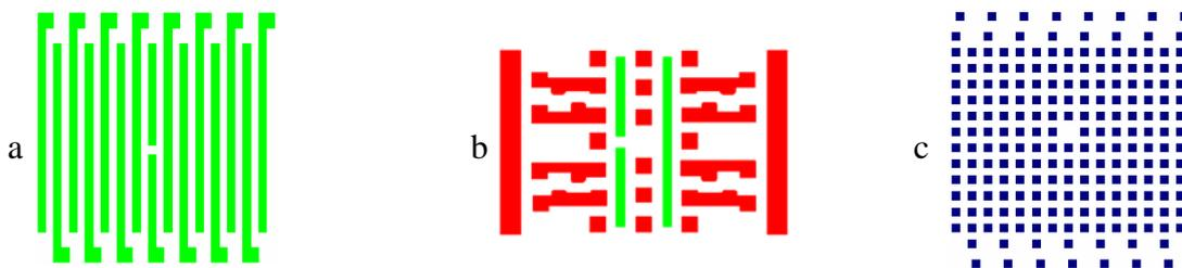
Figure 2. Two types of programmed defects in the layout: a) mousebite defect in the line/space pattern, b) mousebite defect in the SRAM Metal 1 cell, c) missing contact hole defect in the hole array.
