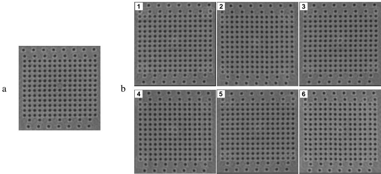
Figure 5. a) SEM image of a missing contact hole defect in the 40nm design before repair. b) SEM images of six identical 40x40nm<sup>2</sup> contact hole defects after repair.
