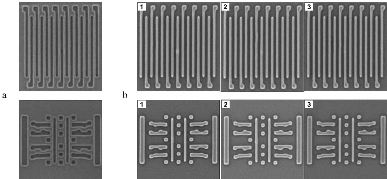
Figure 6. a) SEM images of a repaired 40x50nm<sup>2</sup> mousebite defect in the 40nm line/space and SRAM Metal 1 pattern. b) Imprints of three different repaired defect patterns with identical defect size.
