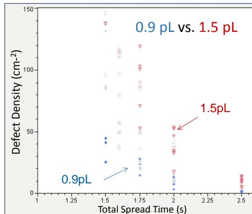
Figure 3. Defect density and spread time improvements when reducing the drop volume from 1.5pL to 0.9pL.
