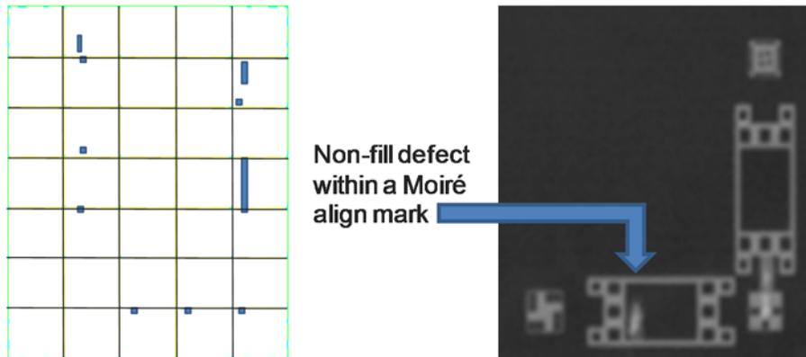
Figure 2. a) Field defect map showing the locations of non-fill defects using a fill time of 1.5 seconds. b) An example of a non-fill defect within a printed Moiré align mark.<sup>13</sup>
