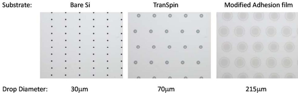
Figure 4. Drop diameter for three different surfaces. A modified adhesion layer promotes fast wetting of the resist.
