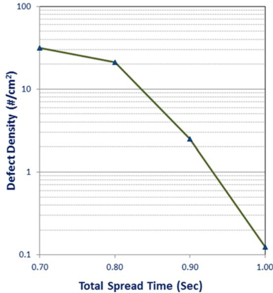
Figure 6. Defect density vs. total spread time. After one second the defect density is close to 0.1/cm<sup>2</sup>.
