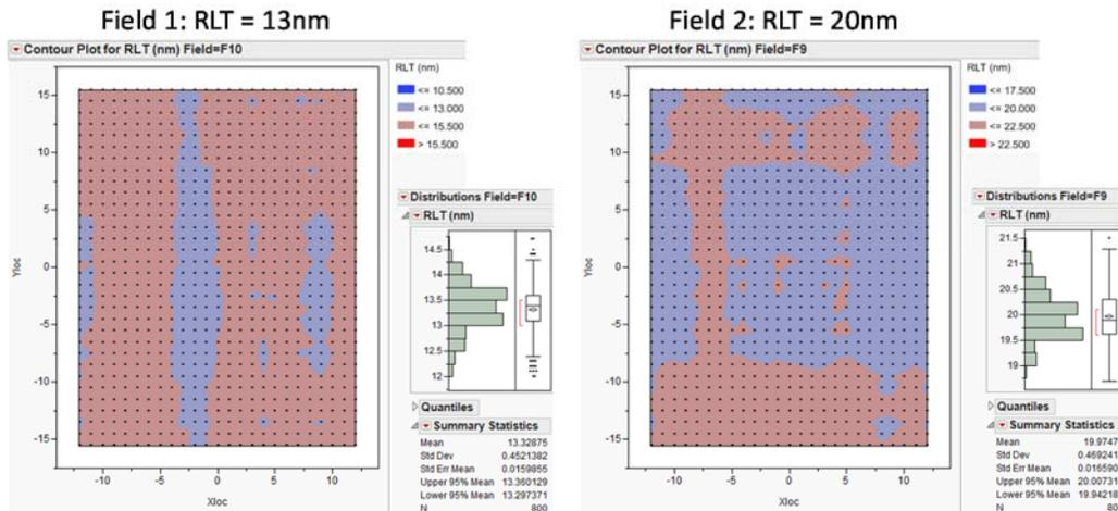
Figure 7. Residual layer thickness uniformity within a field, using 1 pL drop volumes and total resist spread time of 1 second. The in-field variation for both 13 nm and 20 nm was 1.4 nm, 3 sigma.
