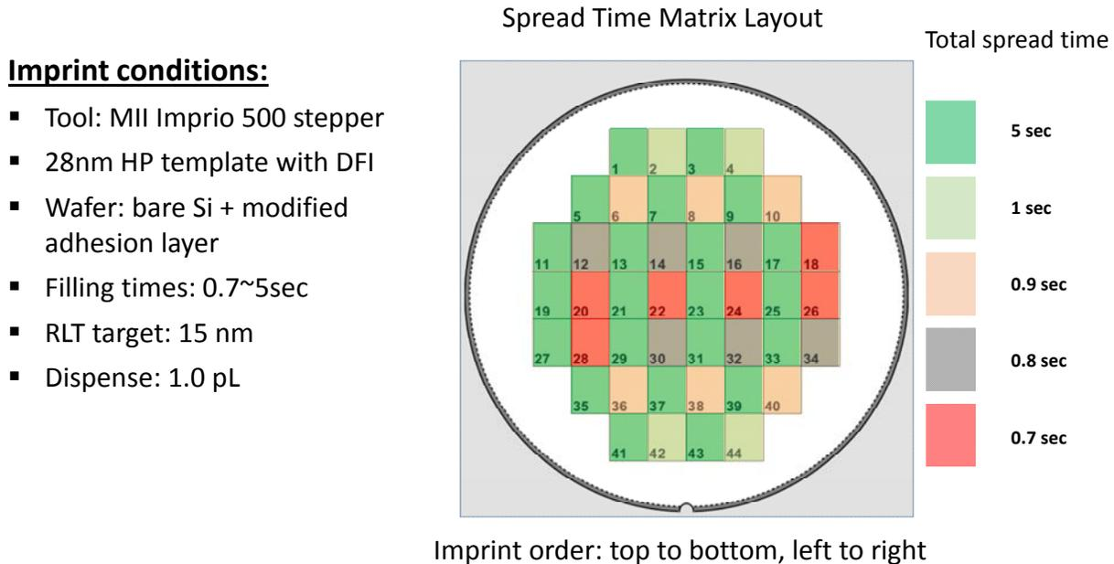
Figure 5. Matrix experiment used to study defectivity as a function of resist spread time.
