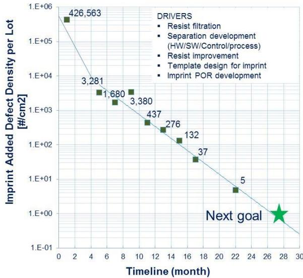
Figure 1. Defectivity reduction to the 5/cm<sup>2</sup> by imprint stepper.
