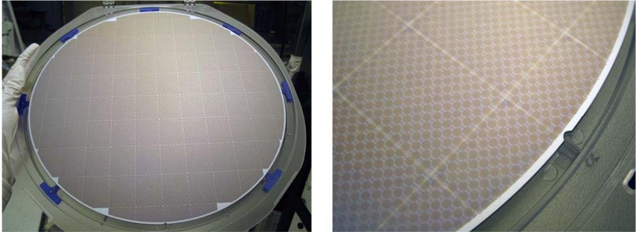
Figure 8. A fully imprinted wafer (left) and a close up of several imprinted edge fields (right).
